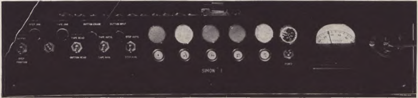
FRONT VIEW of Simon shows its controls and lights. Here the lights show not the answer to a problem but
